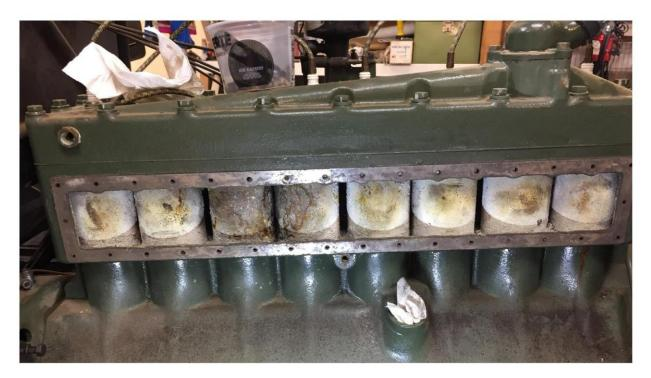
A side note, one of the hazards of running without the distribution plate in place is the the pump discharge may cause accelerated wear of the cylinder walls, see attached photo of how mine looks and it becomes evident where the discharge is right between #5+6. The increased wear caused by the point discharge and maybe some cavitation from running only water as coolant is substantial enough that one cylinder had to be sleeved.
